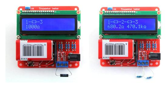
Up to two Resistors are measured and shown with symbols and values with up to four decimal digits in the right dimension. All symbols are surrounded by the probe numbers of the Tester (1-3). So Potentiometer can also be measured. If the Potentiometer is adjusted to one of its ends, the Tester cannot differ the middle pin and the end pin. Resolution of resistor measurement is now up to  $0.01\Omega$ , values up to  $50M\Omega$  are detected.
